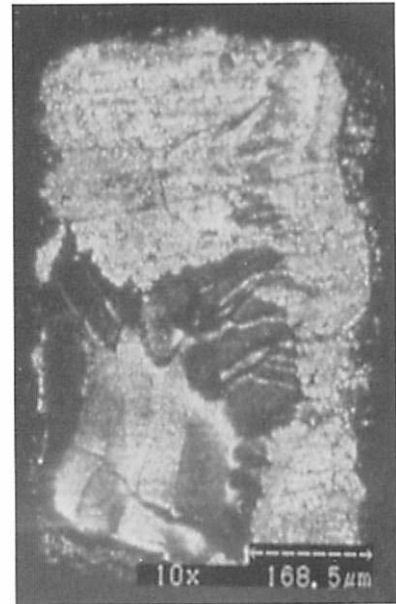
Fig. 4b Lower de-bonded surface of the same beam as 4a. (magnification X250)
